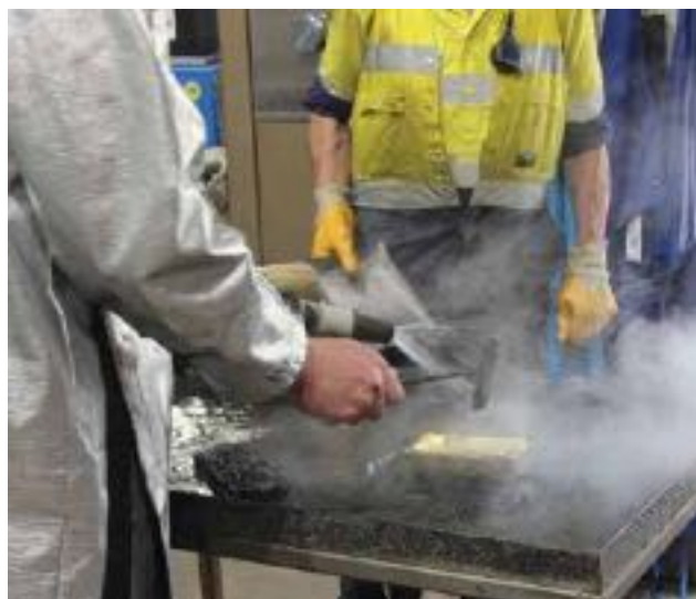
☆ Chipping off the burnt surface of the gold bar.
