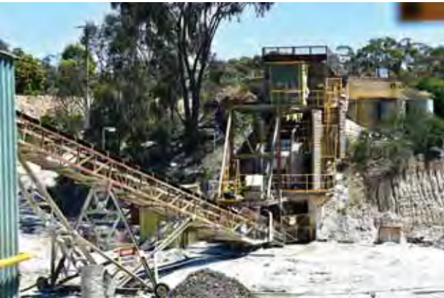
☆ The trucks deposit the ore into the plate feeder, which is then sent through the jaw crusher and onto the radial stacker.
