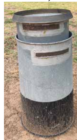
☆ This impressive piece of technology is the Bureau of Meteorology's official rain gauge!
